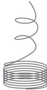
Linear Coils Linear wind, can twist and tangle
