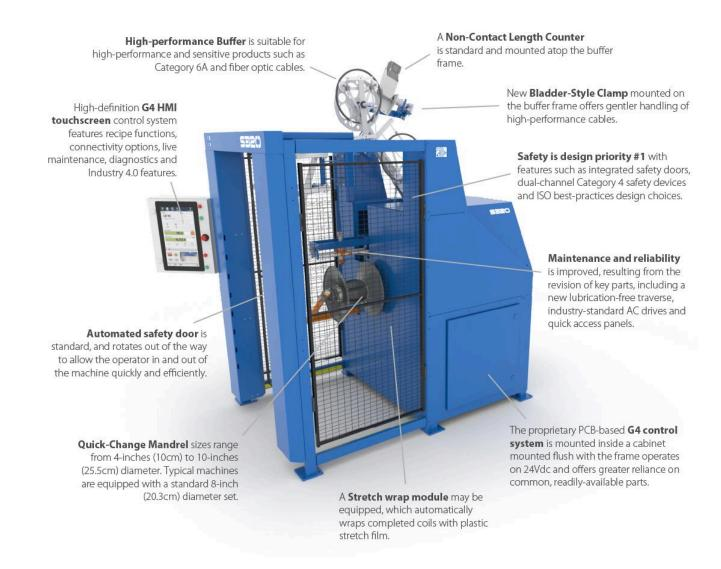
The S320 is REELEX's next-generation single-spindle REELEX coiling machine featuring a variety of new and upgraded components and state-of-the art industrial design.
