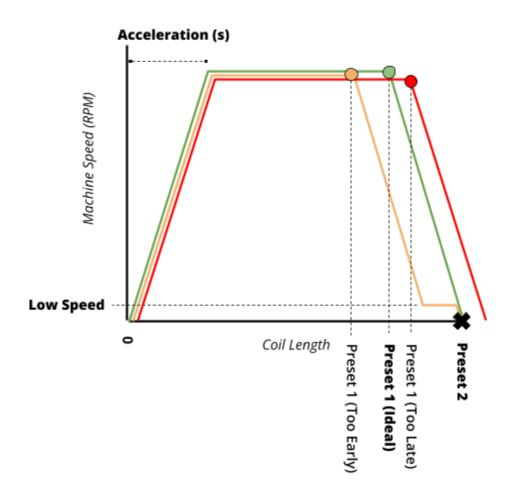
**If Preset 1 is too early** (i.e. too many feet or meters from the end of the coil), the machine will begin to decelerate too soon, and spend too much time at low speed prior to the end of the coil being reached. An early Preset 1 means the machine is not operating as efficiently as it could be, as time spent at low speed should be minimized where possible.
