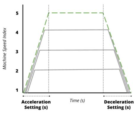
Measured in seconds, this is the time the REELEX machine will take to accelerate to maximum speed or decelerate from maximum speed. This setting sets the rate of acceleration regardless of speed setting.
